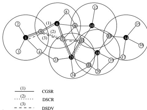
Figure 5: Routing examples (from node 1 to node 11)
