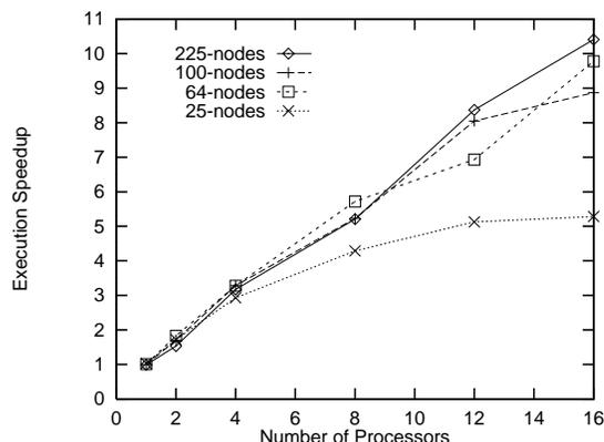
Figure 9: Speedup of parallel simulation in fading channel
