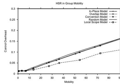
**Figure 11. Control Overhead of HSR vs. Mobility**
