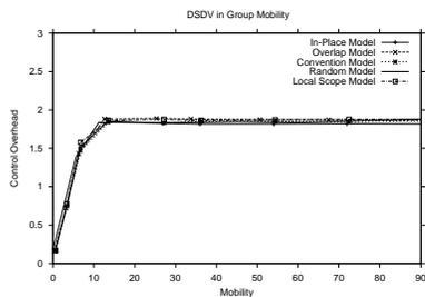
**Figure 10. Control Overhead of DSDV vs. Mobility**
