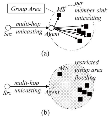
Fig. 1. (a) represents unicasting-based mobile groupcasting, while (b) represents flooding-based mobile groupcasting. Both strategies show inefficient data dissemination when they meet the generic case overall sparse and partially dense.
