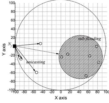
Fig. 3. An example of semi-optimal data delivery within a mobile sink group
